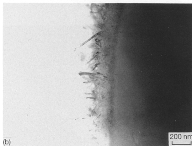
Figure 7 (a) N357, TEM showing carbide at fibre-matrix interface. (b) As (a), showing carbide growth after heat treatment.
